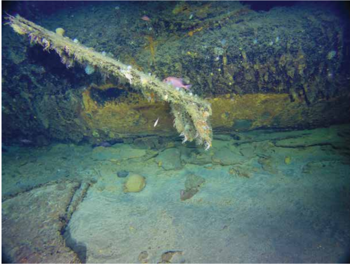
Figure 11 – Pressure hull near starboard after hydroplane, showing concretion delamination. Image courtesy of Paul G Allen, Find AE1 Ltd, Australian National Maritime Museum and Curtin University. © Navigea Ltd
