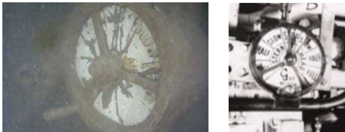
Figure 44 – Conning tower telegraph HMAS AE2 (L), control room telegraph E-Class at build (R). Image courtesy of Paul G Allen, Find AE1, Australian National Maritime Museum and Curtin University. © Navigea Ltd
