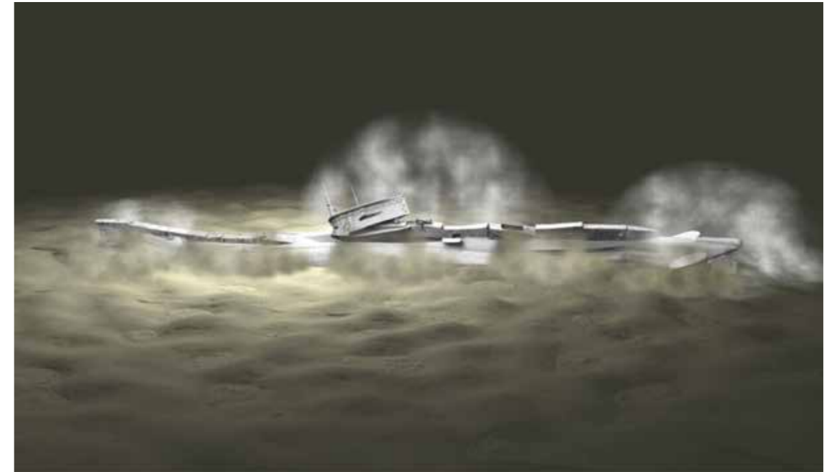
Figure 55 – The hull falls onto its keel, resulting in a third wave of damage, including dislodgement of the hydroplanes and initial dislodgement of the fin. Image courtesy of Paul G Allen, Find AE1, Australian National Maritime Museum and Curtin University. © Navigea Ltd
