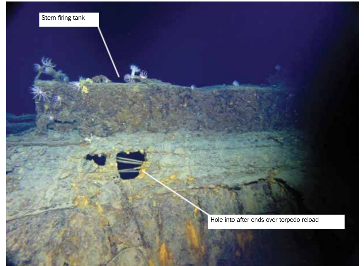
Figure 19 – Stern firing tank and hole over after ends (viewed from port). Image courtesy of Paul G Allen, Find AE1, Australian National Maritime Museum and Curtin University. © Navigea Ltd
