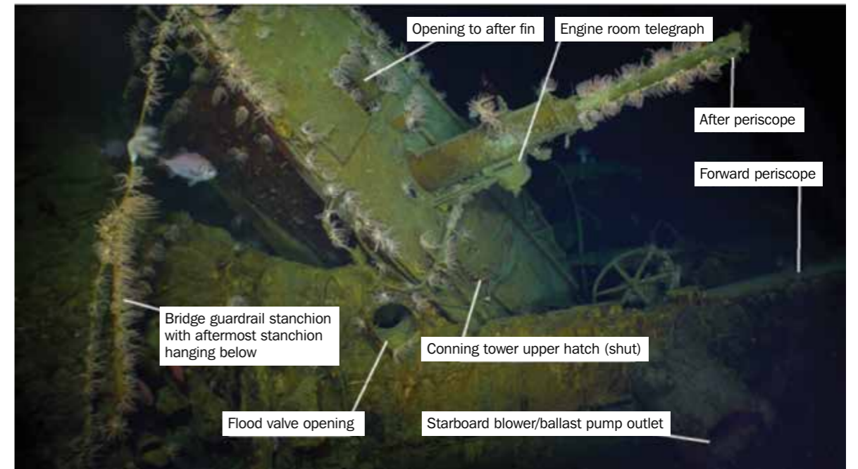
Figure 7 – Fin area from starboard. Image courtesy of Paul G Allen, Find AE1, Australian National Maritime Museum and Curtin University. © Navigea Ltd
