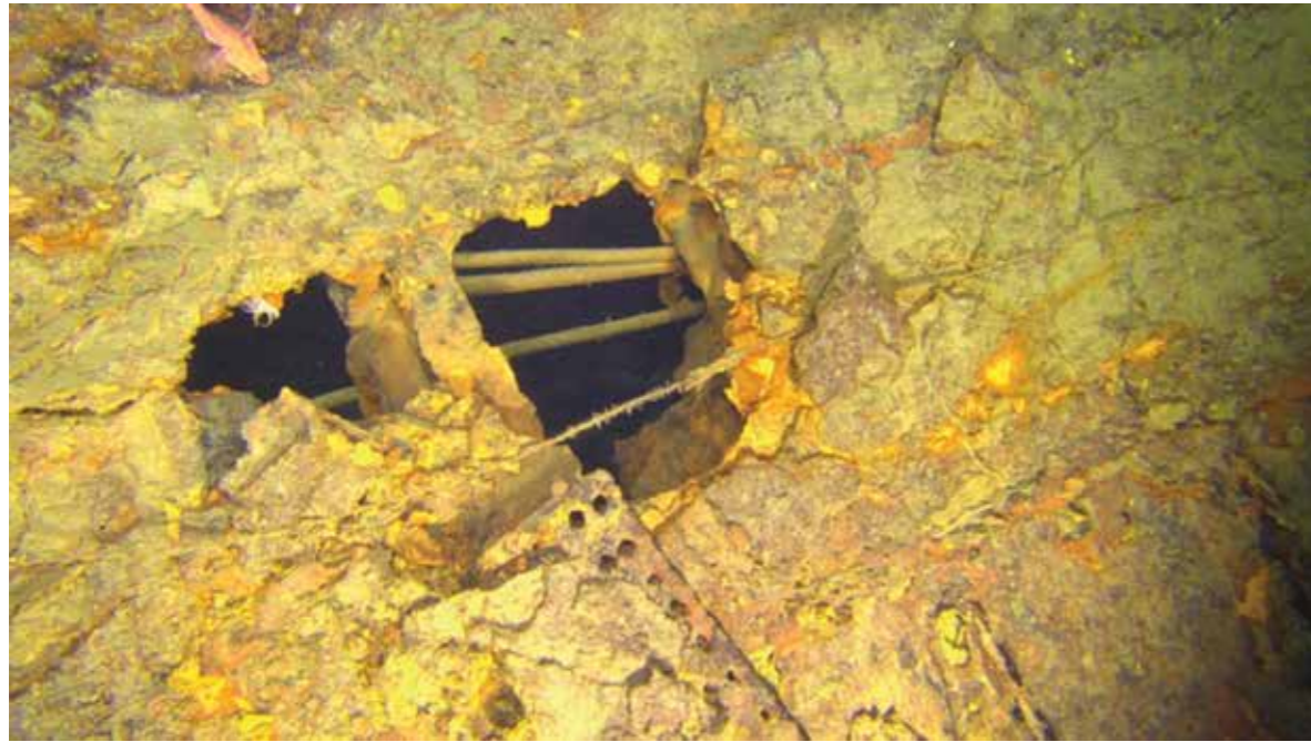
Figure 13 – Hole over senior sailors' mess. Image courtesy of Paul G Allen, Find AE1, Australian National Maritime Museum and Curtin University. © Navigea Ltd
