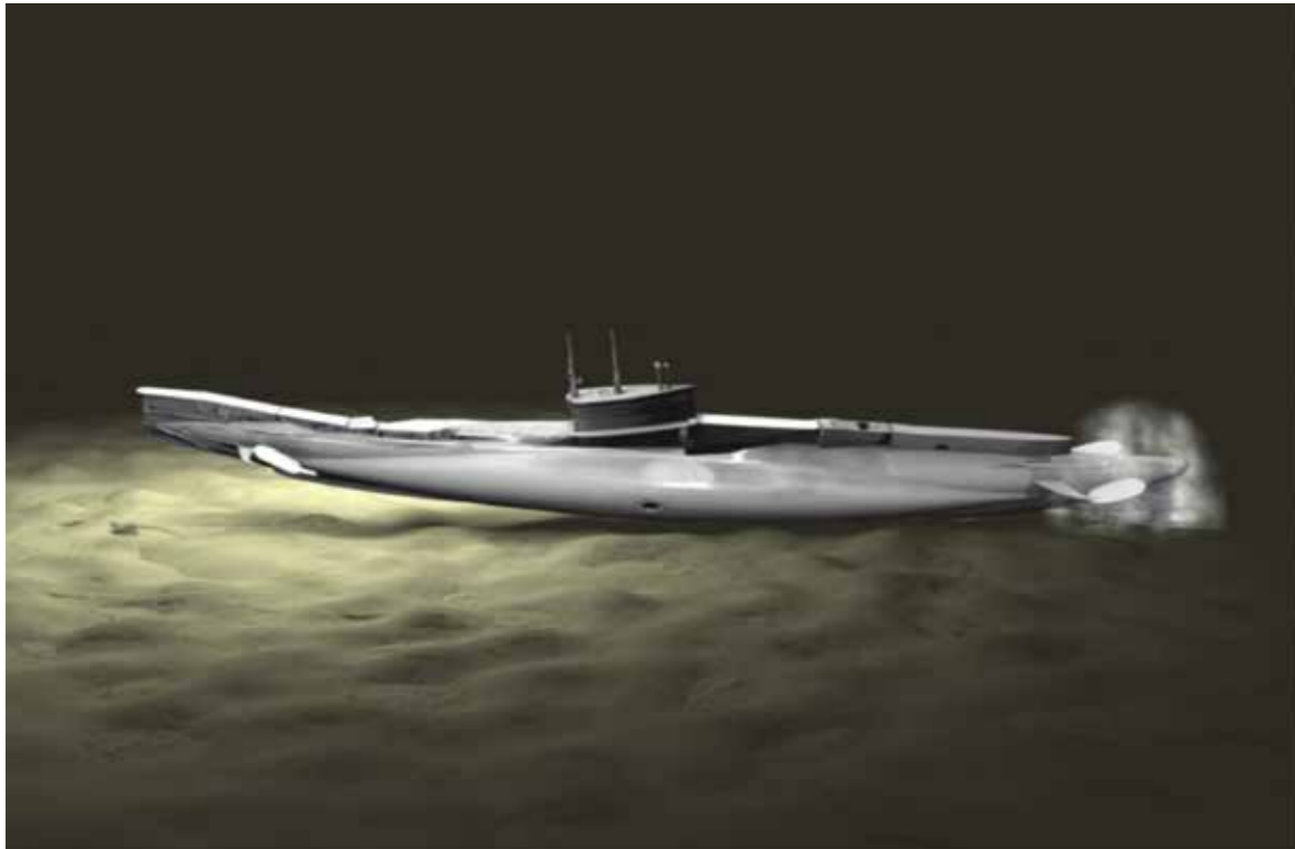
Figure 53 – AE1 continues down, gathering way until she strikes bottom at a bow-up angle of 3–7 degrees, impacting on the rudder and skeg. Image courtesy of Paul G Allen, Find AE1, Australian National Maritime Museum and Curtin University. © Navigea Ltd
