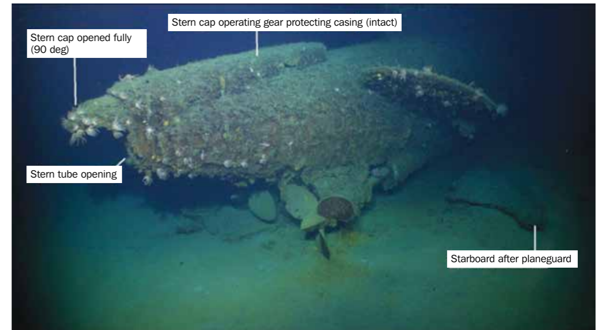
Figure 28 – View of after ends, showing open stern cap. Image courtesy of Paul G Allen, Find AE1, Australian National Maritime Museum and Curtin University. © Navigea Ltd
