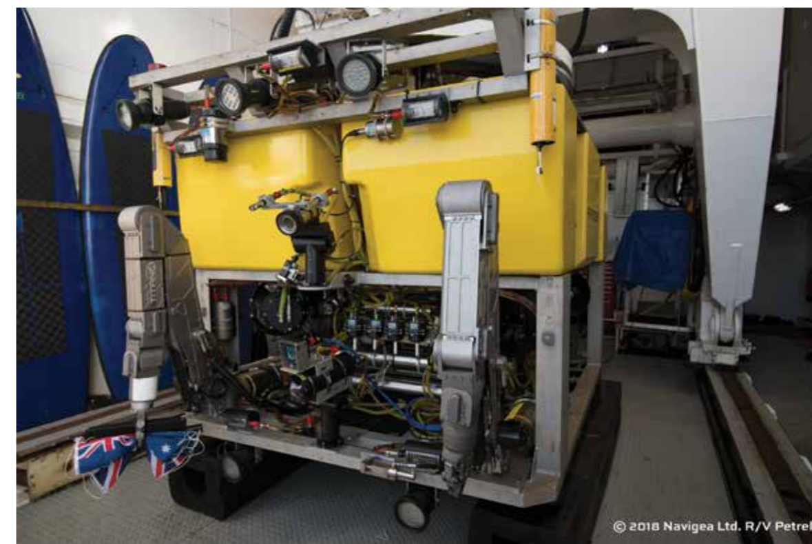
Figure 5 – Triton 6000 remotely operated vehicle. Image courtesy of Paul Mayer
