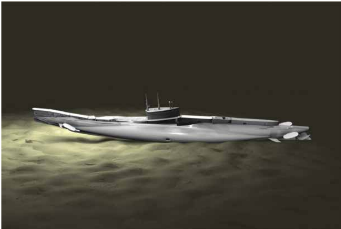
Figure 54 – The skeg and rudder collapse and a second impact occurs on the after end of the keel. Image courtesy of Paul G Allen, Find AE1, Australian National Maritime Museum and Curtin University. © Navigea Ltd
