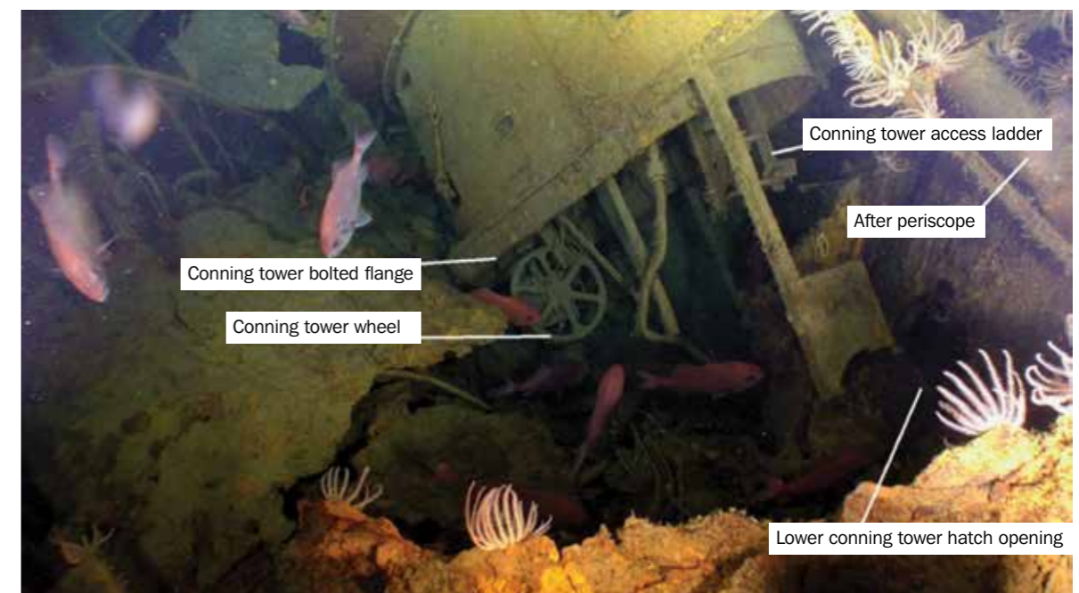
Figure 50 – Underside of toppled fin. Image courtesy of Paul G Allen, Find AE1, Australian National Maritime Museum and Curtin University. © Navigea Ltd
