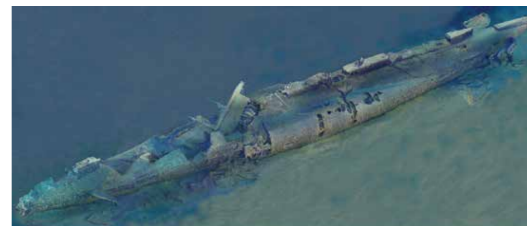
Figure 3 – Interim 3D photogrammetric model of AE1 . The submarine's port side is shown, and the bow is at image left. 3D models by Curtin University from images courtesy of Paul G Allen, Find AE1 Ltd, Australian National Maritime Museum and Curtin University. © Curtin University
