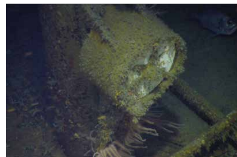
Figure 43 – Engine room telegraph – bridge transmitter. Image courtesy of Paul G Allen, Find AE1, Australian National Maritime Museum and Curtin University. © Navigea Ltd
