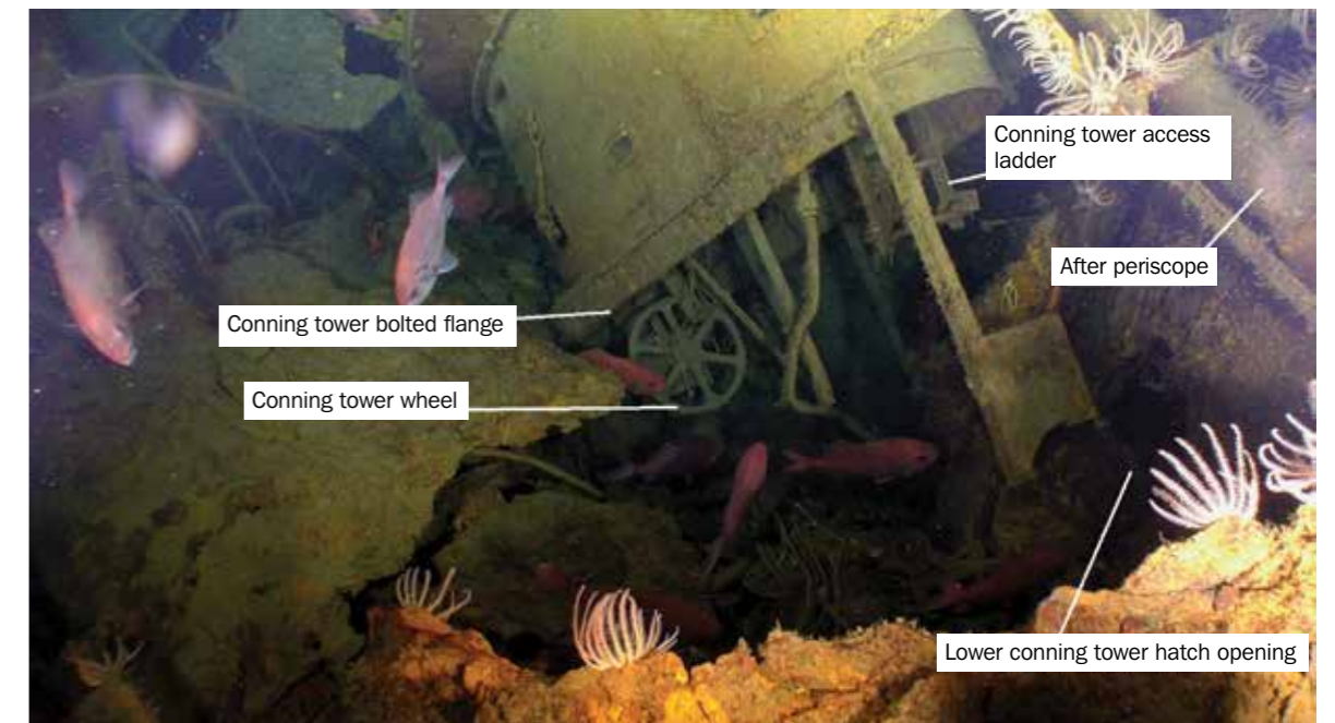
Figure 25 – Conning tower lower hatch opening. Image courtesy of Paul G Allen, Find AE1 Ltd, Australian National Maritime Museum and Curtin University. © Navigea Ltd
