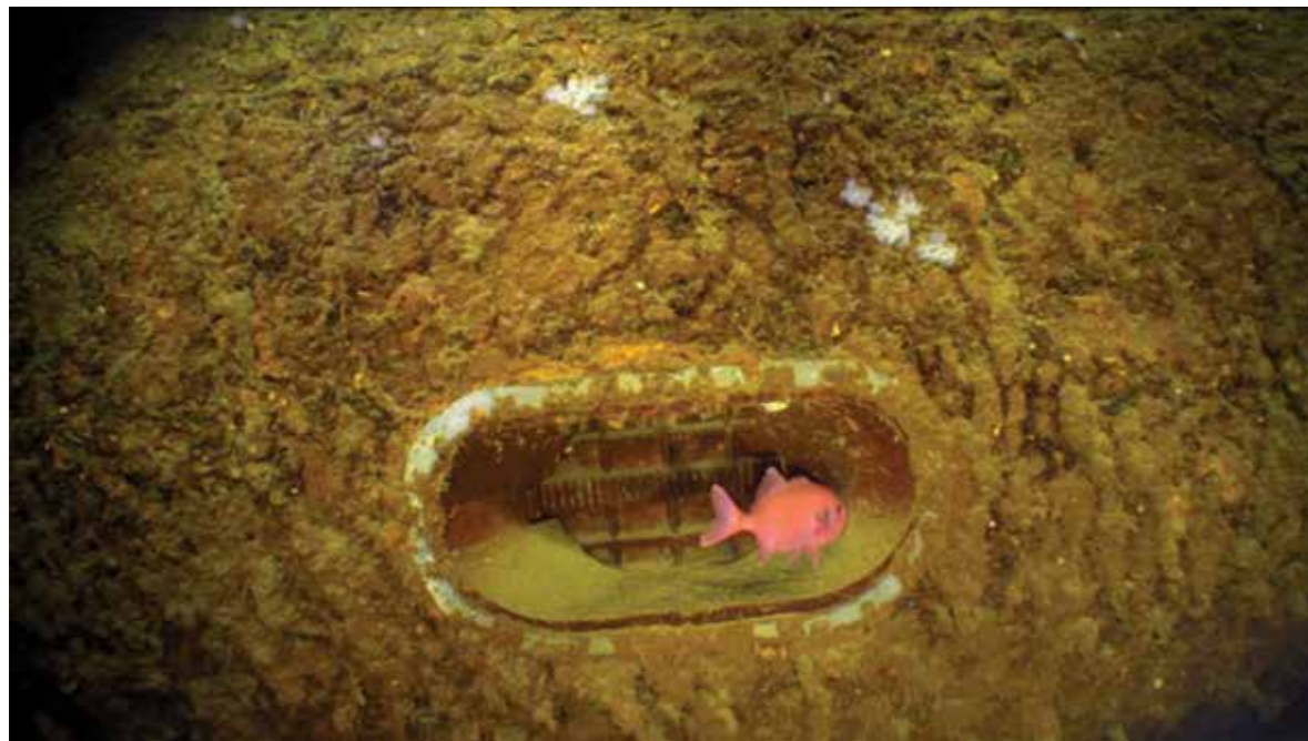
Figure 10 – Starboard beam tube outer door (shut). Image courtesy of Paul G Allen, Find AE1, Australian National Maritime Museum and Curtin University. © Navigea Ltd
