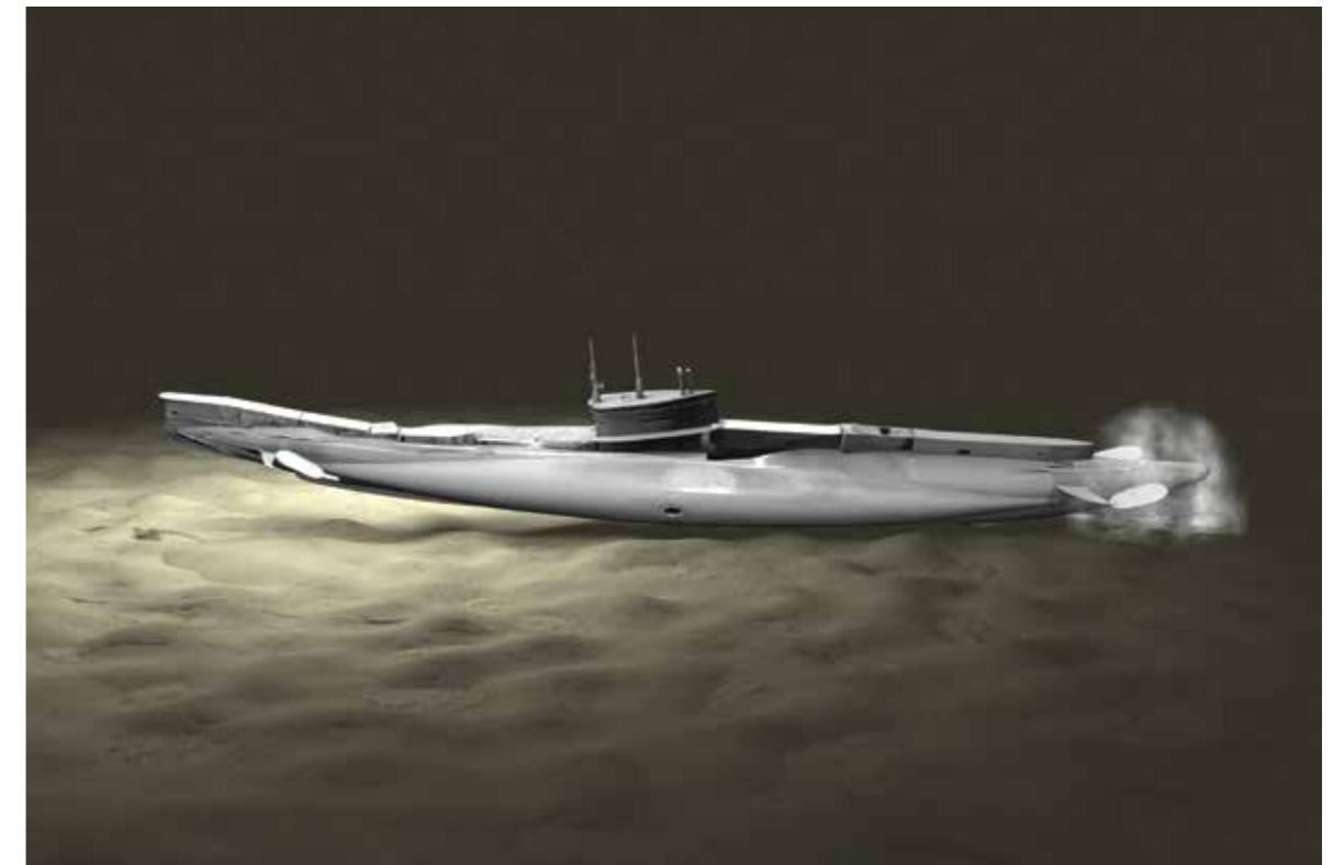
Figure 29 – Artist's impression of the first impact on rudder and skeg. Grant Gittus for Find AE1 Ltd
