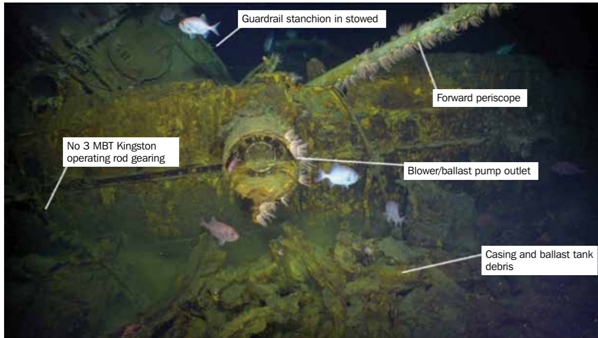
Figure 9 – Starboard blower and No. 3 main ballast tank debris. Image courtesy of Paul G Allen, Find AE1, Australian National Maritime Museum and Curtin University. © Navigea Ltd
