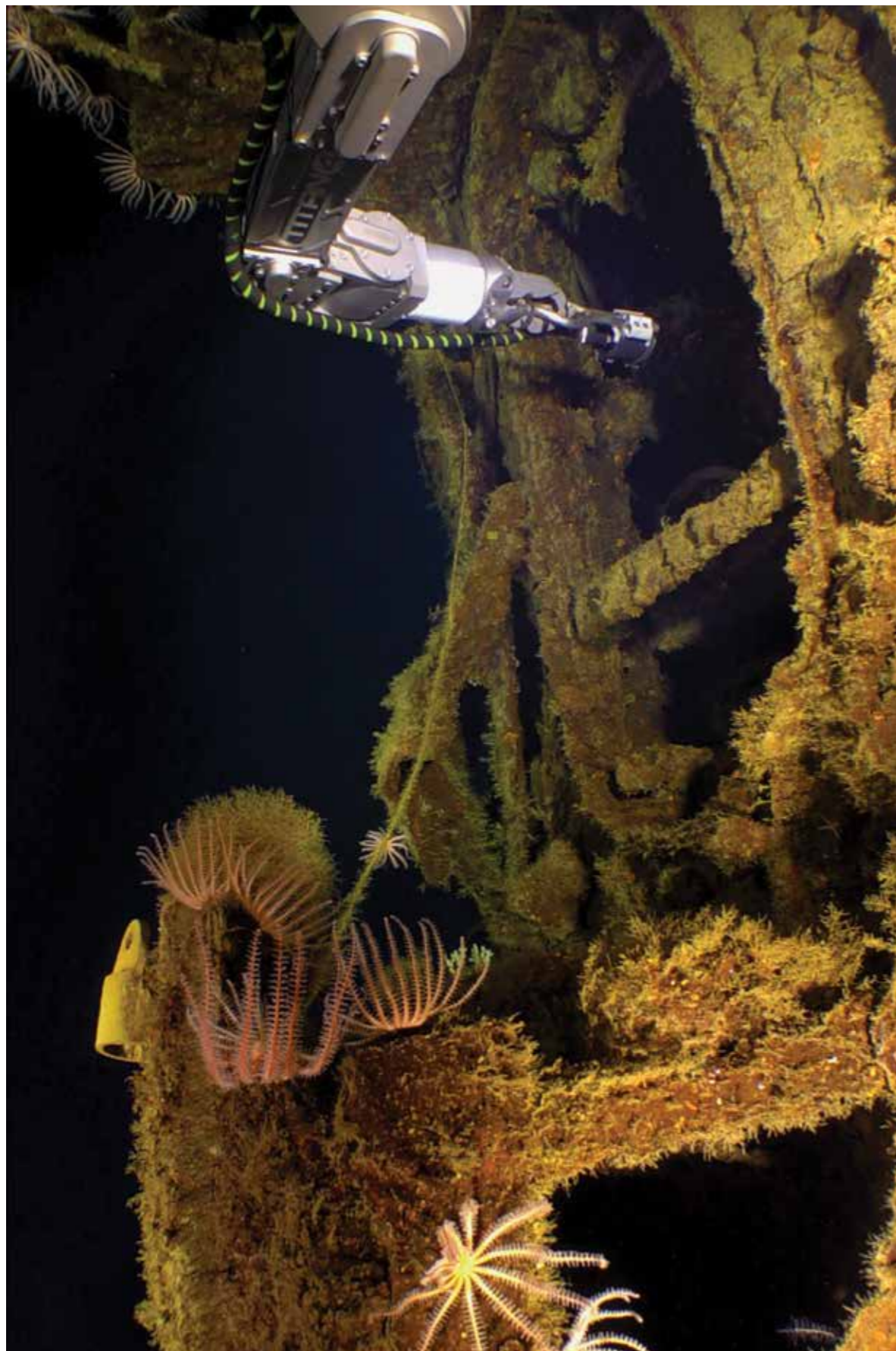
Examining the engine room hatch opening using the ROV's manipulator arm camera. Image courtesy of Paul G Allen, Find AE1 Ltd, Australian National Maritime Museum and Curtin University. © Navigea Ltd
