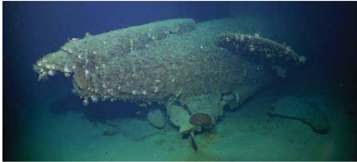
Figure 15 – Protective casing over stern cap operating rod. Image courtesy of Paul G Allen, Find AE1 Ltd, Australian National Maritime Museum and Curtin University. © Navigea Ltd
