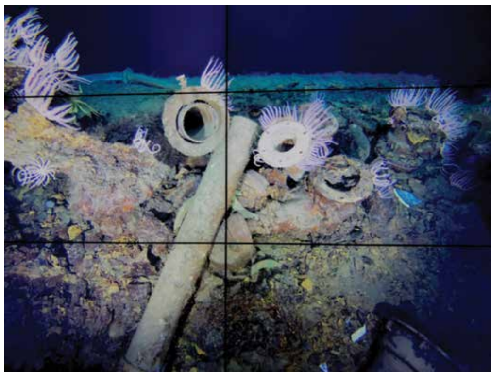
Figure 15 – Image 91-76750, showing debris field of ventilation trunking and flange plates probably associated with waste removal. Image courtesy of Paul G Allen, Find AE1 Ltd, Australian National Maritime Museum and Curtin University. © Navigea Ltd
