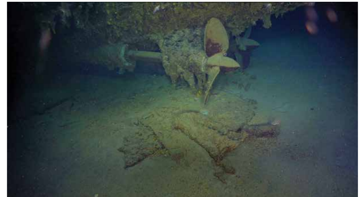
Figure 8 – Displaced rudder and supporting skeg lying under port propeller.
